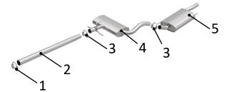
(Carefully read all instructions before installation) Disconnect the vehicle's battery before removal of the OEM exhaust system. This will prevent electrical accidents and will reset the computer if it applies to the vehicle. Remove existing exhaust system from the vehicle. Only remove parts that will be replaced. Clean existing flange with a wire brush to ensure proper sealing.
