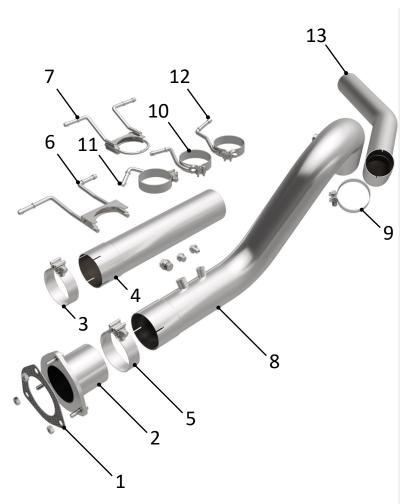
**STEP 1:** (Carefully read all instructions before installation) Disconnect the vehicle's battery before removal of the OEM exhaust system. This will prevent electrical accidents and will reset the computer if it applies to the vehicle. Remove existing exhaust system from the vehicle. Only remove parts that will be replaced. Clean existing flange with a wire brush to ensure proper sealing.
