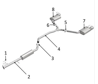
(Carefully read all instructions before installation) Disconnect the vehicle's battery before removal of the OEM exhaust system. This will prevent electrical accidents and will reset the computer if it applies to the vehicle. Remove existing exhaust system from the vehicle. Only remove parts that will be replaced. Clean existing flange with a wire brush to ensure proper sealing.
