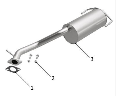
**STEP 1:** (Carefully read all instructions before installation) Disconnect the vehicle's battery before removal of the OEM exhaust system. This will prevent electrical accidents and will reset the computer if it applies to the vehicle. Remove existing exhaust system from the vehicle. Only remove parts that will be replaced. Clean existing flange with a wire brush to ensure proper sealing.
