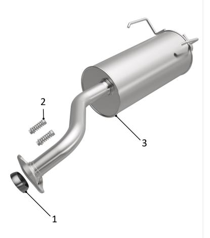
**STEP 1:** (Carefully read all instructions before installation) Disconnect the vehicle's battery before removal of the OEM exhaust system. This will prevent electrical accidents and will reset the computer if it applies to the vehicle. Remove existing exhaust system from the vehicle. Only remove parts that will be replaced. Clean existing flange with a wire brush to ensure proper sealing.
