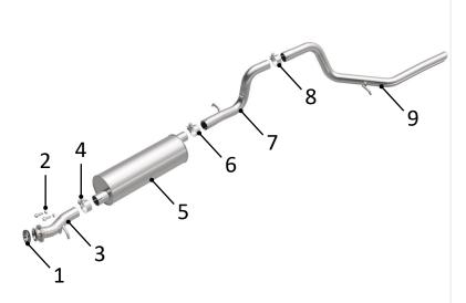
(Carefully read all instructions before installation) Disconnect the vehicle's battery before removal of the OEM exhaust system. This will prevent electrical accidents and will reset the computer if it applies to the vehicle. Remove existing exhaust system from the vehicle. Only remove parts that will be replaced. Clean existing flange with a wire brush to ensure proper sealing.
