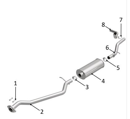
(Carefully read all instructions before installation) Disconnect the vehicle's battery before removal of the OEM exhaust system. This will prevent electrical accidents and will reset the computer if it applies to the vehicle. Remove existing exhaust system from the vehicle. Only remove parts that will be replaced. Clean existing flange with a wire brush to ensure proper sealing.
