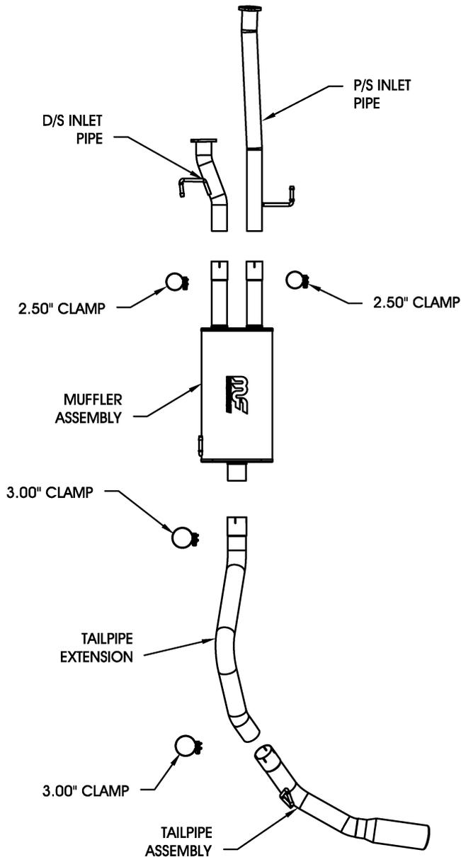
**Step 1:** (Carefully read all instructions before installation) To removed the OEM system unbolt the V-band clamp attaching the tailpipe to the muffler, then unbolt the muffler inlet pipes at the 2-bolt flanges. Do not discard or damage the OEM fasteners or rubber insulators as they will be reused. Disengage the welded hangers from the rubber insulators and remove the muffler and tailpipe.
