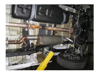
**Step 1.** To remove the OEM exhaust system, you will to need to cut the pipe beind the muffler before it goes over the axle. You can then disengage the welded hangers from the OEM rubber insulators and remove the tailpipe. Unfasten the clamp attaching the OEM muffler inlet to the OEM catalytic converter. Do not damage or discard the OEM fasteners or rubber insulators, as they will be reused to mount the new system. Disengage the muffler hangers and remove the OEM exhaust from the vehicle
