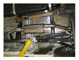
**Step 2.** To begin, fasten the Inlet Pipe Assembly to the catalytic converter using the OEM clamp assembly and by fitting the welded hanger into the OEM rubber insulator (Leave all clamps and fasteners loose for final adjustment of the complete system.) Install the Muffler to the Inlet Pipe Assembly using the supplied 3.00" clamp and fitting the hanger. Next install the Tailpipe Extension to the Muffler in the similar fashion using the supplied 3.00" clamp.
