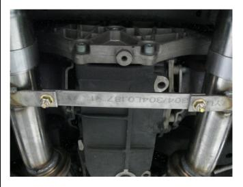
**Step 3.** Next Install the two Resonator and Muffler Assemblies in a similar fashion using the supplied 2.50" clamps and by fitting the welded hangers into the rubber insulators. Attach the supplied cross brace using the included hardware.
