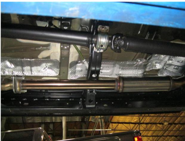
**Step 3.** Begin installation of your new MAGNAFLOW system by attaching the Resonator Assembly to the catalytic converter outlet using the OEM fasteners and insulator. Keep all fasteners and clamps loose until final adjustment.
