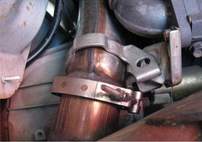
Step 1. Remove the OEM system by first unbolting the the clamp at the outlet of the OEM downpipe and then unbolting the inlet flange of the OEM downpipe from the turbo.
