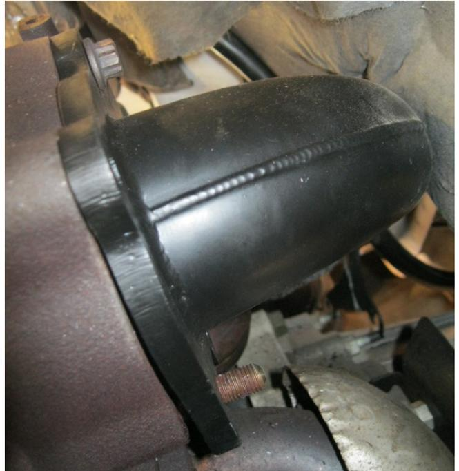
Step 3. Install your new downpipe by first attaching the Inlet flange to the turbo. Using the existing OEM hardware hand tighten the new MagnaFlow downpipe to the Turbo. Then install the clamp onto the outlet and connect to the exhaust system
