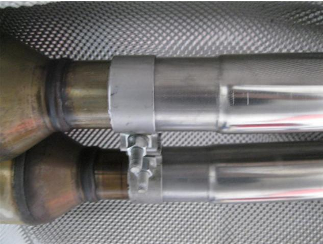
**Step 2.** Begin installation of the new system by slipping the inlet ends of the inlet muffer assembly over the pipes at the catalytic converter that you have just cut. Loosely secure with the supplied clamps.
