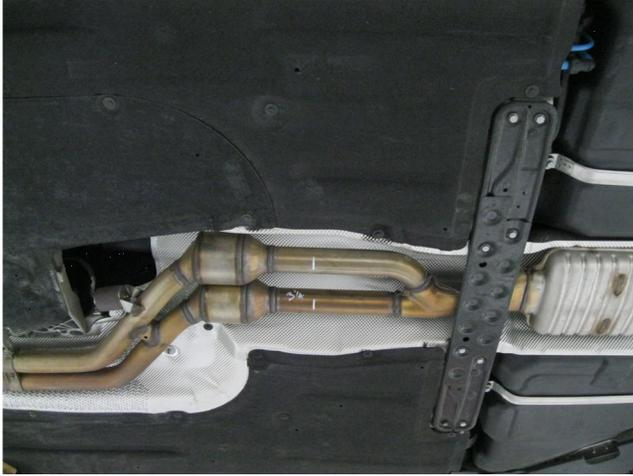
**Step 1.** To allow for extraction of the OEM system you must first remove the underside cross brace. Next cut the two pipes 3.25" behind the catalytic converter welds. Working front to rear detach all hangers from rubber insulators and remove the system. Retain rubber insulators and clamp as they will be re-used to mount the new system.
