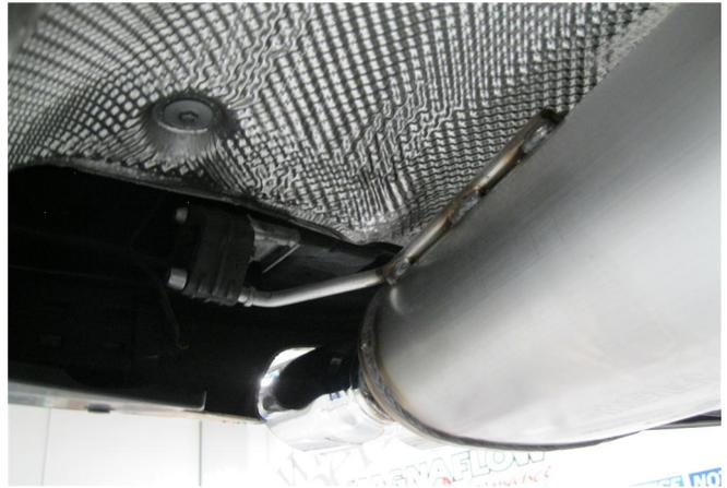
**Step 3.** Next attach the Tail Pipe Muffer Assembly to the Inlet Muffer Assembly using supplied clamp and fit hangers into rubber insulators. Re attach cross brace.
