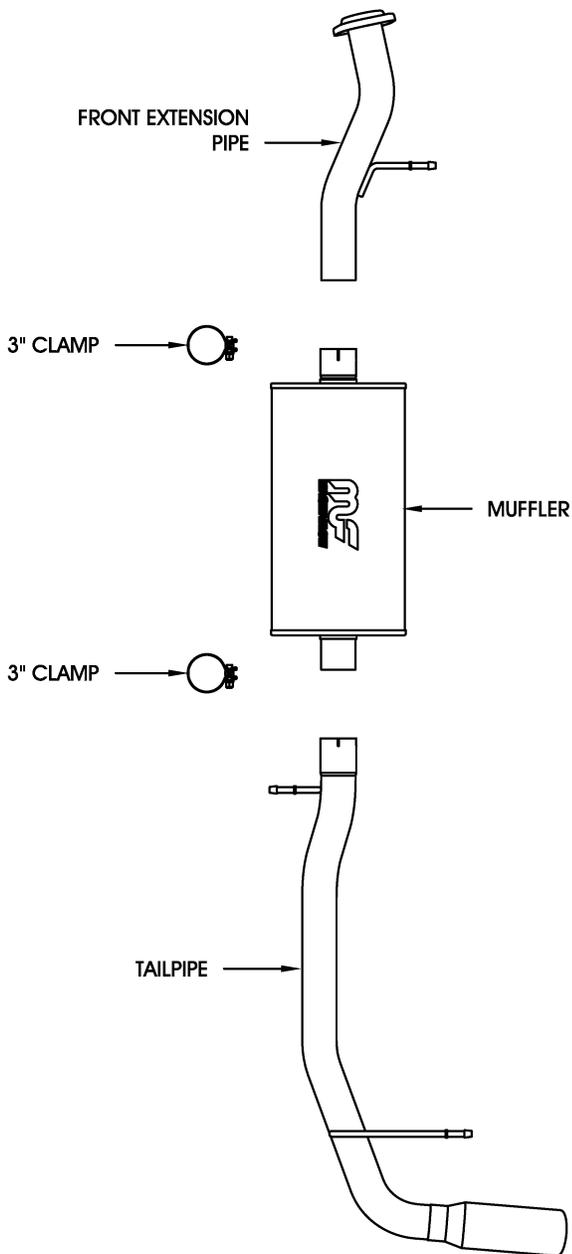
**Warning:** When working on under or around any vehicle exercise caution. Please allow the vehicle's exhaust system to cool before removal, as exhaust system temperatures may cause severe burns. If working without a lift, always consult vehicle manual for correct lifting specifications. Always wear safety glasses and ensure safe work area. Serious injury or death could occur if safety measures are not followed.
