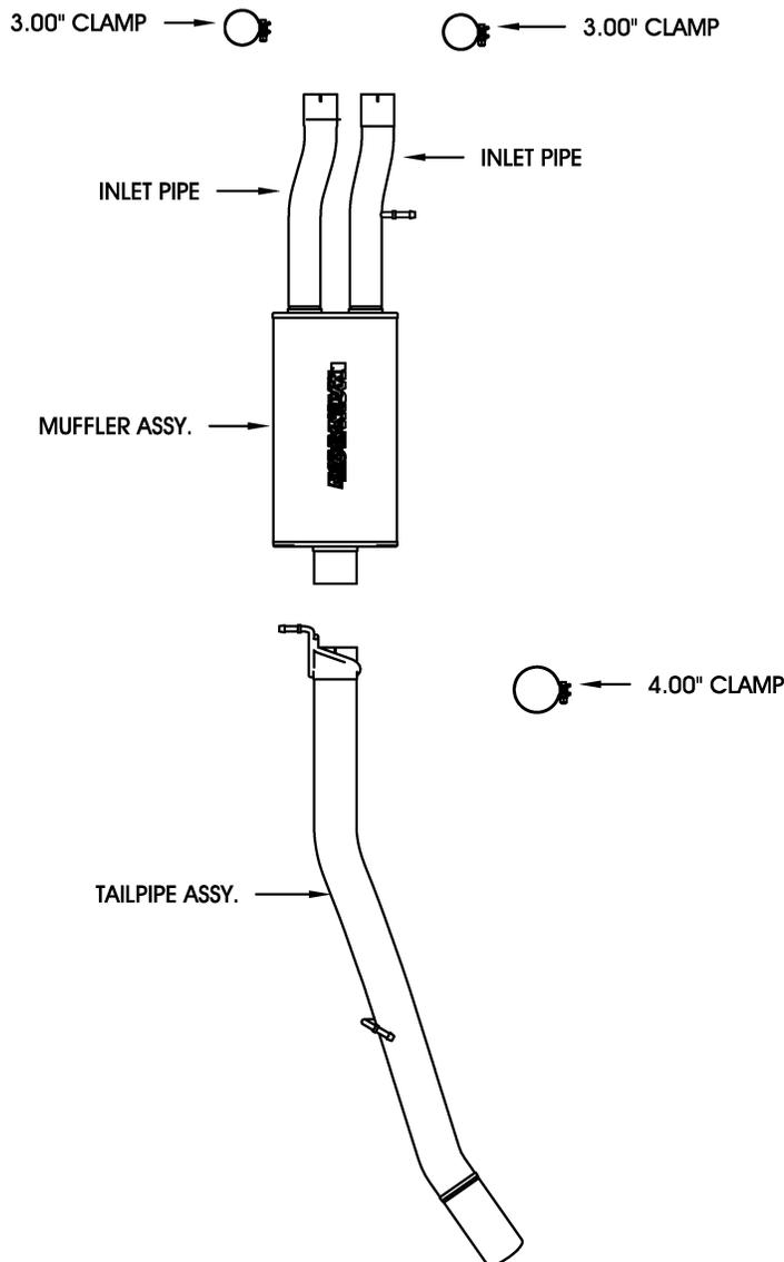
**Step 1:** (Carefully read all instructions before installation) To remove the OEM exhaust system, measure 12" from the front of the muffler forward and cut the catalytic converter extension pipes. You may need to cut the tail pipe to aid in removal. Remove the exhaust from the OEM rubber insulators. Do not damage the OEM rubber insulators, as they will be re-used to mount the new system.
