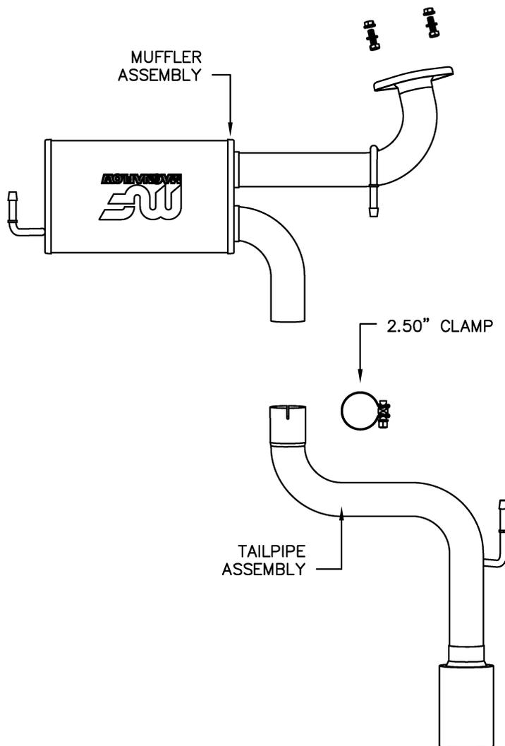
**Step 1:** (Carefully read all instructions before installation) To remove the OEM muffler assembly, unbolt it at the 2-bolt flange and disengage the welded hangers from the OEM rubber insulators to extract it from the vehicle (Do not damage the OEM rubber insulators, as they will be reused to mount the new system).
