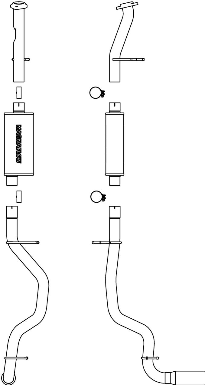
**Step 1:** (Carefully read all instructions before installation) To remove the OEM exhaust system, unbolt the muffler inlet pipe from the catalytic converter at the 2-bolt flange (Do not discard the OEM fasteners, as they will be re-used to mount the new system). Disengage the welded hangers from the OEM rubber insulators and remove the system from the vehicle. Raising the rear end of the vehicle with a jack, or cutting the exhaust system will aid in removal.
