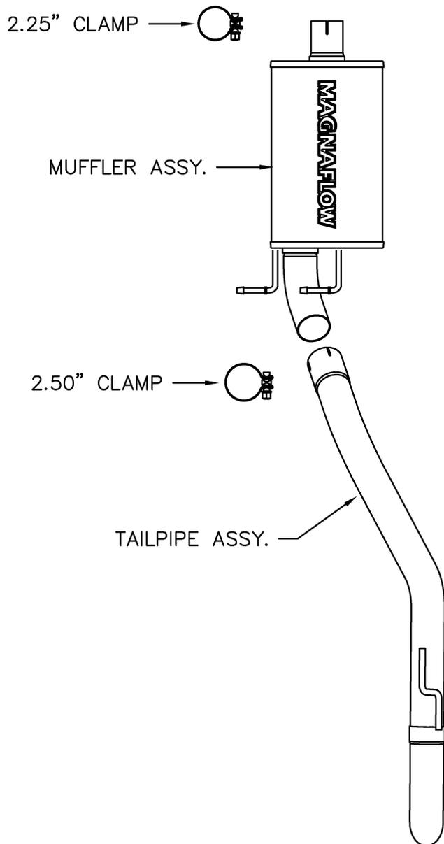
**Step 1:** (Carefully read all instructions before installation) Disconnect the vehicle's battery before removal of the OEM exhaust. This will allow the computer to reset itself with the new system, and prevent electrical accidents. To remove the OEM system, unbolt the muffler and tailpipe at the mating connections, disengage the welded hangers from the OEM rubber insulators, and remove the assemblies. Do not damage the OEM rubber insulators, as they will be reused to mount the new system
