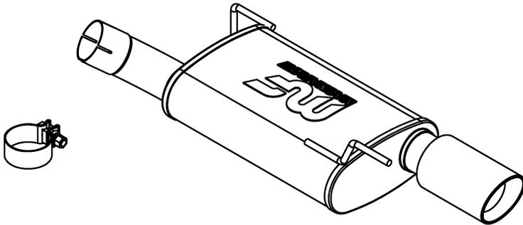
**Step 2:** Before installing the new muffler assembly, slide the supplied 2.50" clamp onto the inlet pipe. Install the new muffler assembly by fitting the welded hangers into the rubber insulators, and by fastening the muffler inlet to the over-axle pipe using the supplied clamp. Be sure to line up the large notch in the inlet pipe with the alignment peg on the over-axle pipe, or the muffler will not fit properly.
