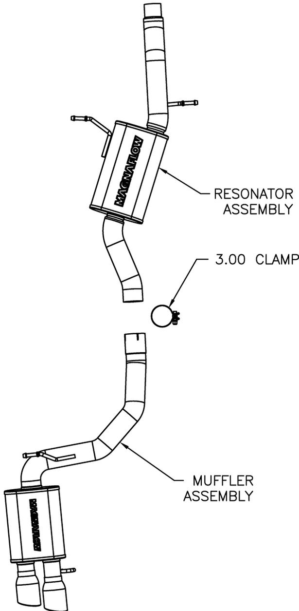
**Step 1:** (Carefully read all instructions before installation) Begin removal of the OEM exhaust by loosening the OEM clamp located behind the front Resonator Assembly. Working front to rear disengage the welded hangers from the rubber insulators and extract the exhaust system from the vehicle. Do not discard the OEM clamp or damage the rubber insulators, as they will be used to mount the new system
