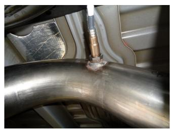
Step 7. For 6.7L models remove the O2 sensor plug from the Over Axle Pipe and attach the O2 sensor.
