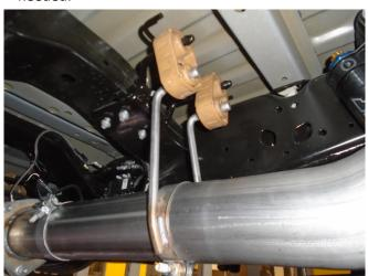
Step 4. Begin the installation by loosely attaching the Inlet Pipe Assembly to the OEM flange outlet using the OEM hardware (6.7L), or loosely attaching the Inlet Adapter to the DPF outlet using the supplied clamp (6.4L). Loosely attach the Extension Pipe, if needed, using the supplied clamp.
