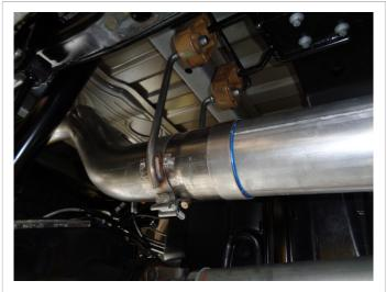
Step 5. Loosely slip Hanger Clamp Assy #1 over the inlet end of the Over Axle Pipe Assembly and locate the hangers to the rubber insulators. Loosely install the Over Axle Pipe Assembly using the supplied clamp.
