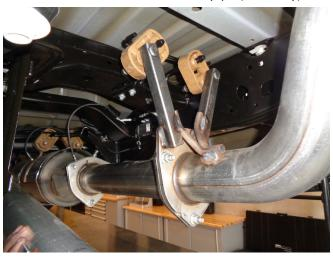
Step 2. Next, Unbolt the extension pipe assembly from the DPF outlet flange (6.7L) or loosen the band clamp attaching the inlet pipe (6.4L). Working front to rear disengage all welded hangers from the rubber insulators. Be sure to retain all mounting hardware as it will beneeded to install your new MAGNAFLOW system.
