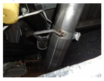
Step 6. To install the Tail Pipe Assembly loosely slip the Hanger Clamp Assembly over the pipe inlet. #2 for model years up to 2017, #3 for model years 2017 and up. Loosely secure using the supplied clamp and engaging the welded hanger to the rubber insulator.
