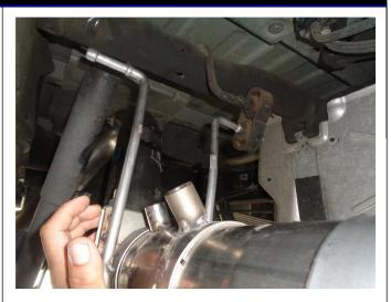
**Step 2. 2014-2020 Installation:** Begin installation of the Magnaflow system by clamping the extension pipe to the newly cut outlet of the DPF using the supplied 4.00" clamps and fitting the hangers in the rubber insulators (leave all clamps loose for final adjustment of the complete system). If your vehicle has any sensor(s) re-install at the appropriate locations. Any boss that doesn't get a sensor installed into it must be closed off with a provided screw in plug.
