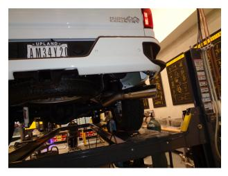
**Step 4.** Once a final position has been chosen for the new exhaust system, evenly tighten all clamps and fasteners, from front to rear, using the torque specifications on page one of the instructions. Inspect all fasteners after 25-50 miles of operation and re-tighten if necessary.
