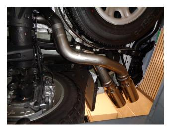
**Step 3.** Complete the installation by sliding the specified Rear Hanger Clamp Assy onto the Tailpipe Assy and attaching the Tailpipe Assy to the Over Axle Pipe. Engage the hangers into OE rubber insulators.
