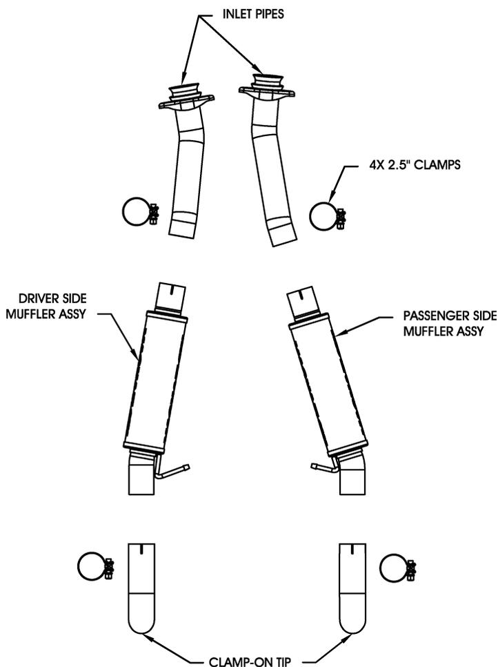
**Step 1:** To begin removal of your OEM exhaust system, you will need to cut the tail-pipes just behind the mufflers. Remove the tail pipes from the OEM rubber insulators. Do not damage the rubber insulators, as they will be re-used with your new system. Next unbolt the extension pipes from the H-pipe and remove the mufflers from their OEM rubber insulators. Do not discard the fasteners required to bolt the extension pipes to the mufflers, as they will be re-used.
