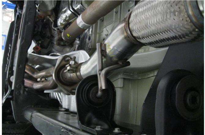
**Step 4.** Locate the welded hangers to the rubber isolators. Working front to rear use a similar technique to install the Pipe Extension, Muffler Assembly and Tip.
