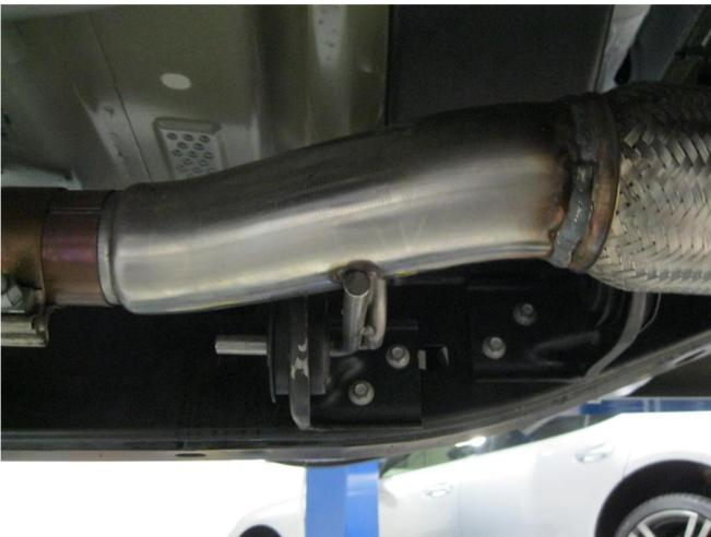
**Step 3.** Begin installing your new system by attaching the inlet pipe assembly to the catalytic converter outlet pipe. Loosely secure using the OEM clamp.
