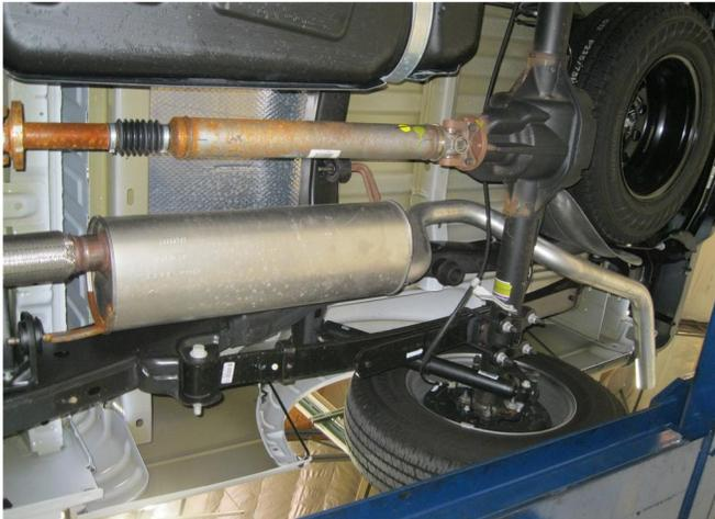
**Step 2.** Working front to rear loosen all connecting band clamps. Carefully remove the welded hangers from the rubber isolators. The OEM system can now be removed. Be sure to retain all mounting hardware as it will be needed to install your new MAGNAFLOW performance exhaust system.
