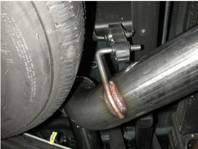
**Step 5.** With all components mounted loosely, adjust the system for overall aesthetics and clearance of frame & bodywork. (MAGNAFLOW recommends at least 1/2" of clearance between the exhaust system and any body panels to prevent heat-related body damage or fire.)
