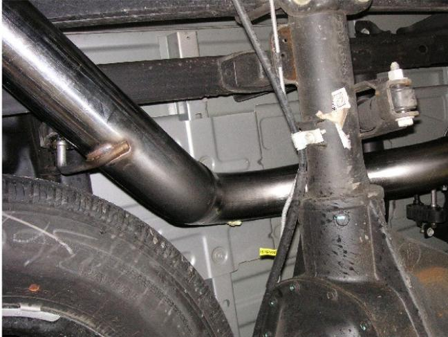
**Step 4.** Loosely install the Over Axle Pipe and Tail Pipe Assembly using the supplied Hanger Clamps. The Outlet may be trimmed as desired.
