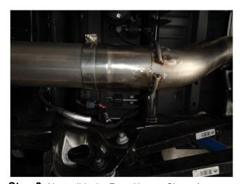
**Step 3.** Next, slide the Front Hanger Clamp Assy loosely onto the Over Axle Pipe Assy then attach Over Axle Pipe Assy to the Inlet Pipe using the supplied 5.00" Clamp. Engage the hangers into the rubber insulators. (Leave all clamp and fasteners loose for final adjustment of the complete system.)
