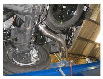
**Step 4.** Complete the installation by sliding the Rear Hanger Clamp Assy onto the Tailpipe Assy and attaching the Tailpipe Assy to the Over Axle Pipe. Engage the hangers into OE rubber insulators.
