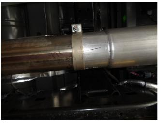
Step 2. Your vehicle configuration will determine which length of inlet pipe is used. See the table below for the cut point of the supplied extension pipe. The dimensions are the length of pipe you will need for your application. Begin installation of the MagnaFlow system by attaching the appropriate Inlet Pipe to the outlet of the DPF using the supplied 4.50" clamp.
