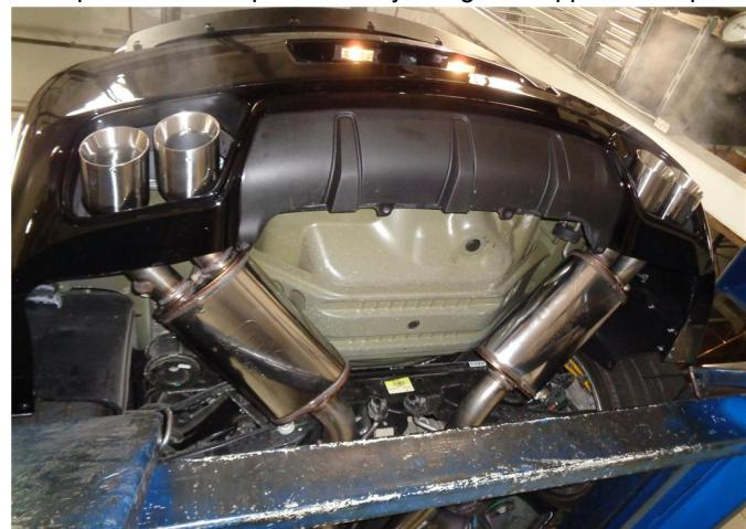
**Step 4.** Loosely install both muffler assemblies using the supplied clamps. Locate all welded hangers to the OEM rubber insulators.
