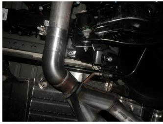
**Step 4.** Loosely install both Tailpipe Assemblies using the supplied clamps. Locate all welded hangers to the OEM rubber insulators.
