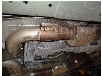
**Step 1.** To remove the OEM exhaust system you will first need to loosen the clamps attaching it to the catalytic converter outlet pipes, then working front to rear (with the exhaust supported) disengage all welded hangers from the rubber insulators. The OEM exhaust system can now be removed. Retain all mounting hardware as it will be needed to install your new MAGNAFLOW system.
