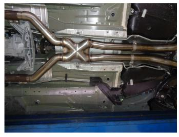
**Step 2.** Begin installing the new system by loosely attaching the inlets of the X-Pipe Assembly to the catalytic converter outlets using the OEM clamps.
