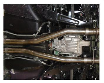
**Step 3.** Next, loosely install both driver and passenger side Mid Pipes to the X-Pipe Assembly using the supplied clamps.
