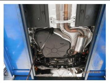
**Step 3.** Begin installing the new system by inserting the inlet of the Resonator Assembly into the clamp at the outlet of the OEM exhaust and fitting the hangers into the rubber insulators. Leave clamp loose for final adjustment.
