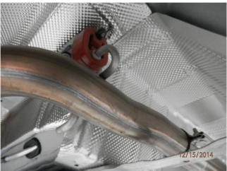
**Step 2.** Once cut, begin removing the exhaust by loosening the factory clamp located in front of the resonator. Working rearward extract the hangers from the rubber insulators (retain clamp and insulators as they will used in the installation of the new exhaust system). Remove the OEM system from the vehicle.
