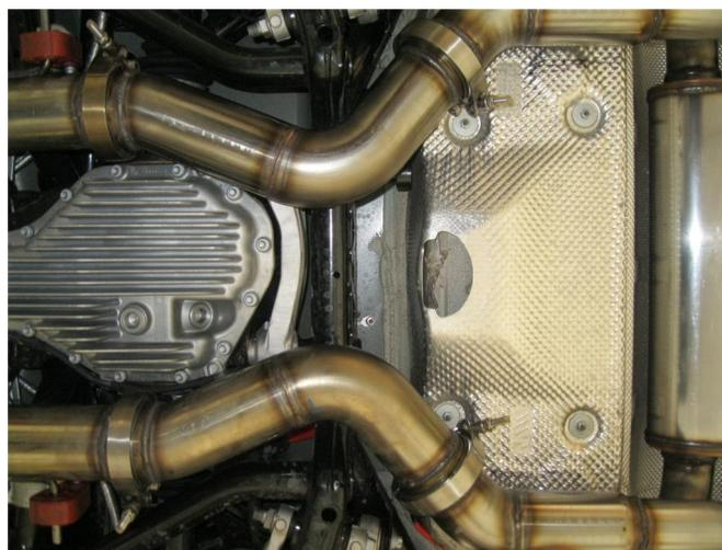
**Step 4.** Loosely Install the D/S and P/S Mid Pipe Assemblies with the supplied V-Band Clamps.
