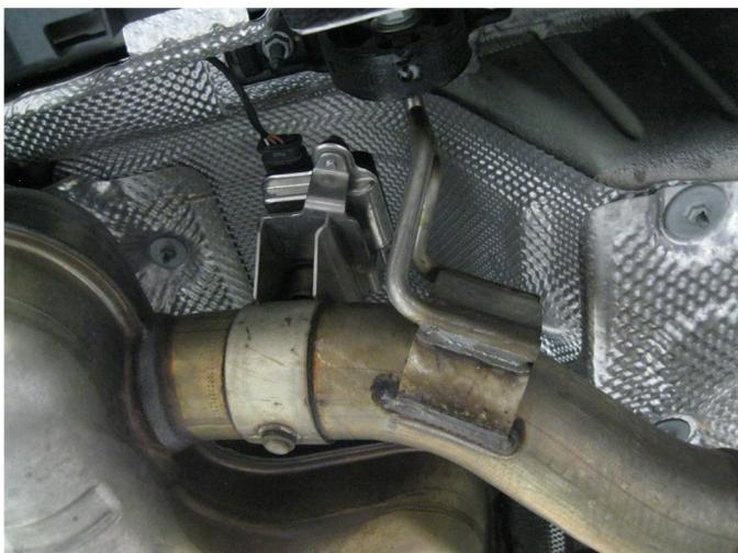
**Step 1.** To remove the OEM exhaust system you will first need to unplug the exhaust valve control motors located on the OEM muffer assembly.
