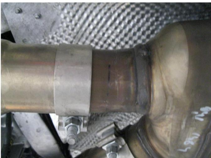
**Step 2.** You will need to cut the two outlet pipes 4.00" rearward of the underbody muffer. Disengage all welded hangers from the OEM rubber insulators. Do not discard the OEM fasteners or damage the rubber insulators as they will be needed to mount your new MAGNAFLOW system. Once the OEM system has been removed you can unbolt the two exhaust control valves located on the muffer assembly.
