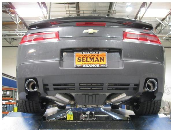
**Step 4.** Once a final position has been chosen for the new exhaust system, evenly tighten all clamps from front to rear using the torque specifications on page one of the instructions. Inspect all fasteners after 25-50 miles of operation and re-tighten if necessary.
