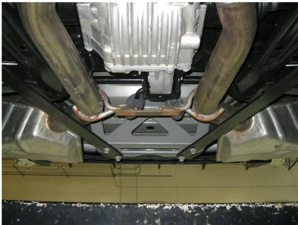
**Step 1.** Begin by removing the two rear chassis stiffeners by the muffler inlets. This will allow access to the exhaust system.
