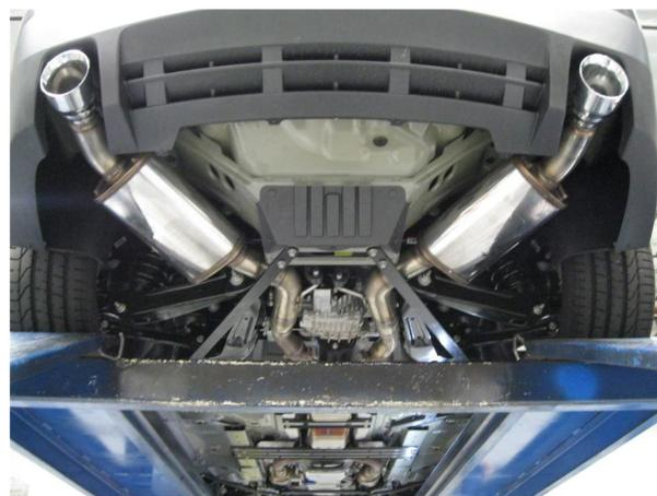
**Step 3.** Install the new system by attaching the Driver and Passenger Muffler Assemblies to the cut portion of the OEM system using the supplied 3.00" clamps. Leave clamps loose for final adjustment. Fit the hangers into the rubber insulators.
