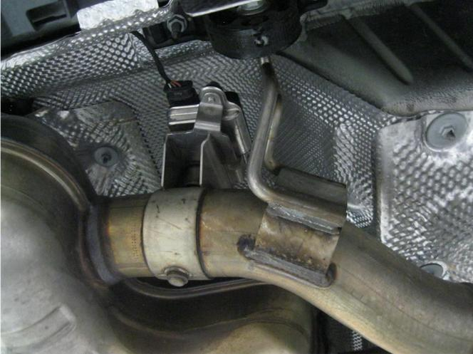
**Step 1.** To remove the OEM exhaust system you will first need to unplug the exhaust valve control motors located on the OEM muffler assembly.
