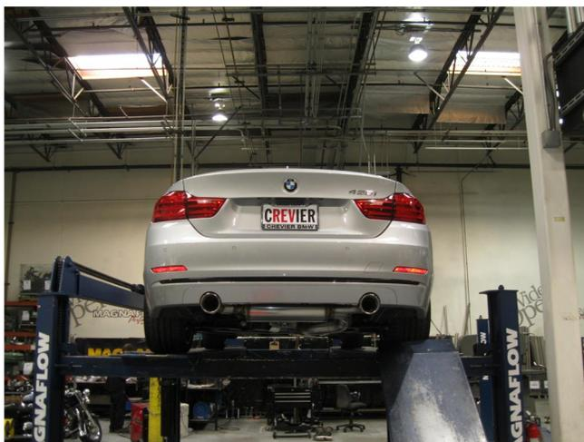
**Step 6.** Once a final position has been chosen for the new 6system, evenly tighten all clamps from front to rear using the torque specifications on page one of the instructions. Inspect all fasteners after 25-50 miles of operation and re-tighten if necessary.
