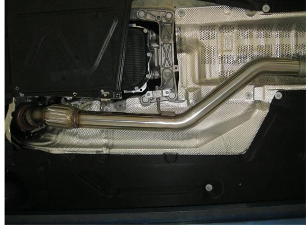
**Step 3.** Begin installation of the new system by fastening the Inlet Pipe Assembly to the outlet of the catalytic converter using the OEM v-band clamp and fitting the hanger into the rubber insulator.
