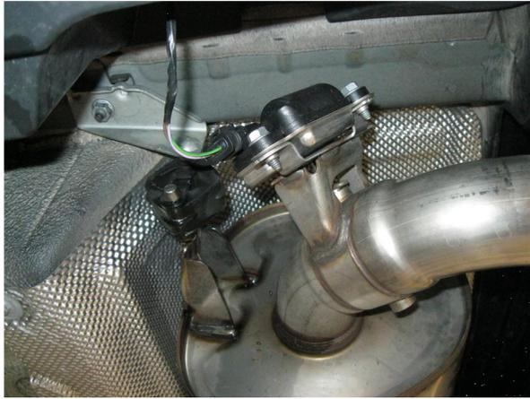
**Step 1.** To remove the OEM exhaust system you will need to remove the cross braces/stiffener and unplug the electronic exhaust control valve at the rear of the vehicle . Start by loosening the v-band clamp at the catalytic converter junction, working rearward disengage the hangers from the rubber insulators (retain rubber insulators and OEM v-band clamp) and remove the OEM system.
