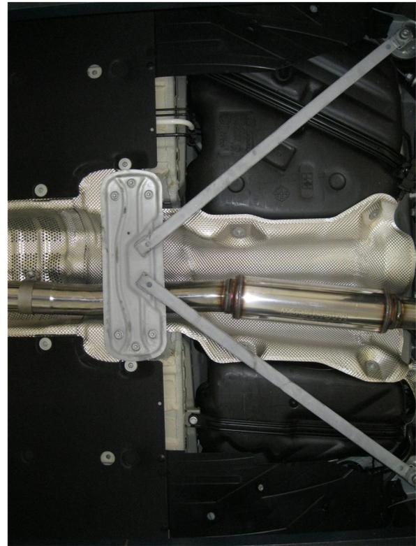
**Step 4.** Next fasten the Resonator Assembly to the inlet pipe using the supplied 3.00" clamp.
