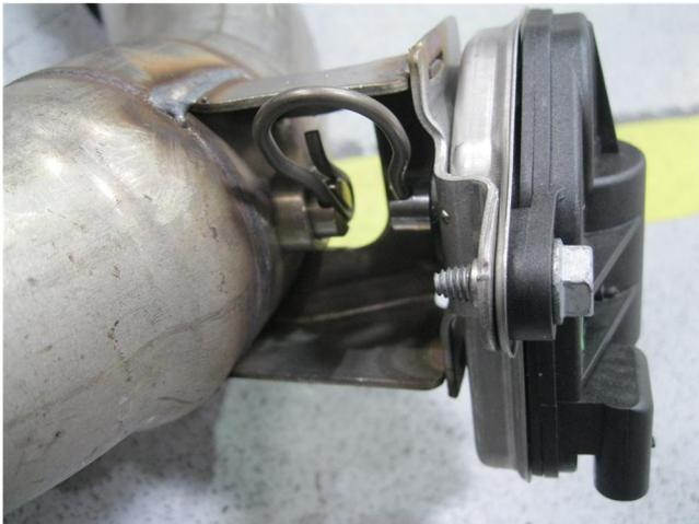
**Step 2.** Once on the OEM system is on the ground you will need to swap the servo motor from the factory control valve to the control valve on the Magnaflow Muffler Assembly. Unbolt the motor and remove the drive spring (take notice of how the drive spring is orientated as it must be re-installed the same way) and steel heat shield. Install the motor and heat shield to the valve, insert the drive spring and tighten.
