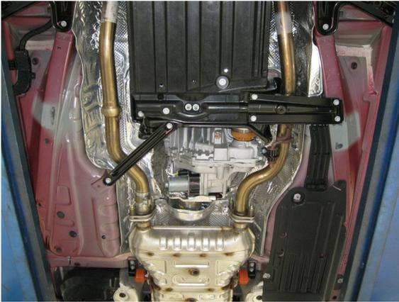
**Step 1.** Begin removal of the OEM exhaust system by unfastening the spring loaded two bolt flanges located in front of the factory resonator.
