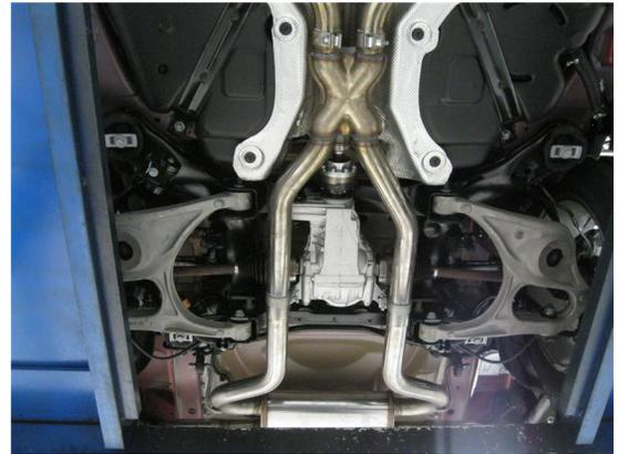
**Step 4.** Next use the supplied 2.50" clamps to attach the X-Pipe to the Resonator Assemblies.
