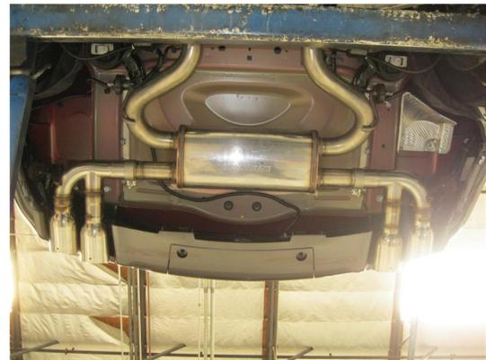
**Step 5.** Finish by attaching the Muffler Assembly to the Mid Pipe and the Tail Pipe Assemblies to the Muffler using the supplied 2.50" clamps. Fit hangers into rubber insulators.
