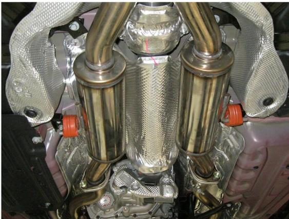
**Step 3.** Begin installation of your new MAGNAFLOW system by attaching the Driver and Passenger side Resonator Assemblies at the two bolt flange locations using the supplied 10MM bolts and the OEM nuts and springs and fitting the hangers into the rubber insulators. Keep all fasteners and clamps loose until final adjustment.
