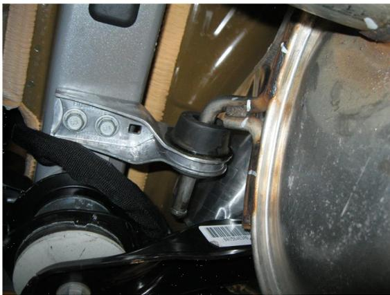
**Step 2.** Working rearward disengage the hangers from the rubber insulators and un-fasten the two bolt flange at the driver side rear muffler and remove the OEM exhaust.
