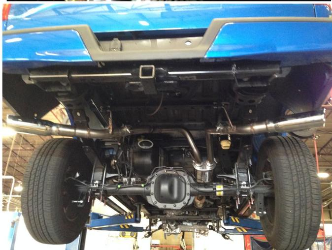
**Step 5.** To allow for the installation of a dual outlet system on a single outlet vehicle you will have to mount the supplied Hanger Brackets to existing holes in the factory frame rails using the supplied fasteners (8mm bolt and panel nut) as shown in the photos. Once completed you can now slide the Tailpipe assemblies onto the Over Axle pipes and fasten with the supplied 2.50" clamps and mount the hangers to the installed hanger brackets using the supplied rubber insulators.
