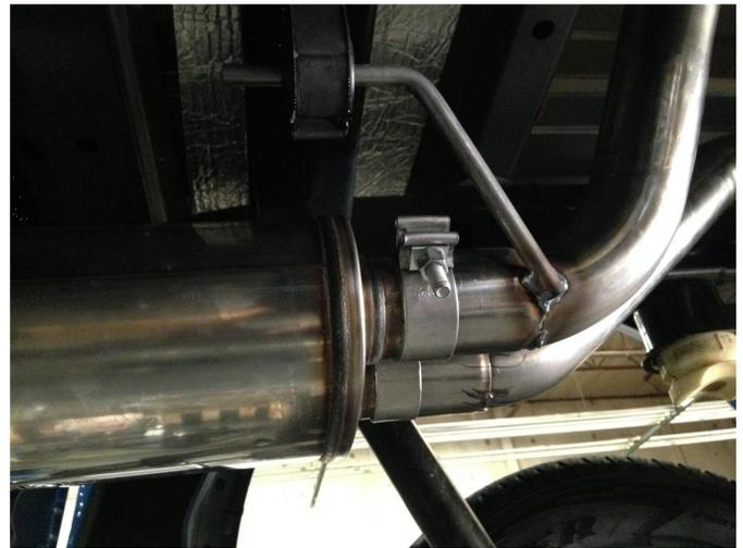
**Step 4.** Install both the Over Axle Pipes using the supplied 2.50" clamps. Locate the welded hanger to the OEM rubber insulator.
