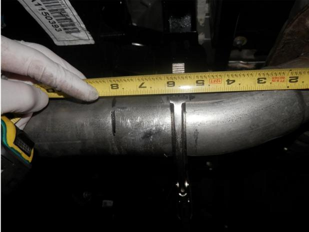
**Step 1.** It is necessary to cut the factory exhaust system to install the new Magnaflow unit. To do this measure 5.75" in front of the welds on the rear muffler inlets. Deburr the cut pipes to facilitate installation of the new system.
