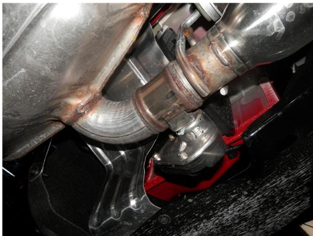
**Step 2.** Next you will need to unplug the electrical connection on the rear Exhaust Valve Control Motors (Qty 2) located on the OEM exhaust assembly.
