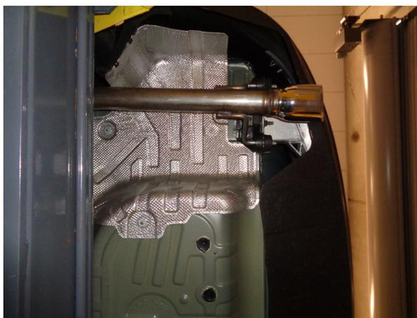
Step 3: Next loosely fasten the Extension Pipe to the Resonator Assembly using the supplied 2.25" clamp. Then attach Tail Pipe Assembly in a similar fashion engaging the welded hangers to the rubber insulators.
