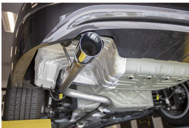
Step 4: Once a final position has been chosen for the new exhaust system, evenly tighten all clamps from front to rear using the torque specifications on page one of these instructions. Inspect all fasteners after 25-50 miles for operation and re-tighten if necessary.
