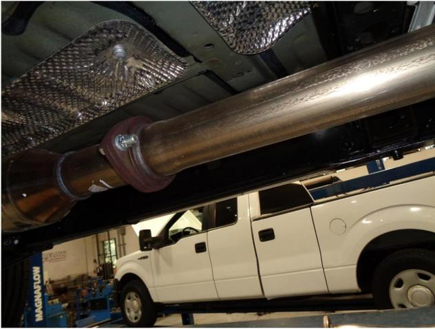
**Step 1.** Begin removal of the OE system by unfastening the flange attaching the exhaust to the catalytic converter. Do not discard or damage the OE fasteners or rubber insulators as they will be used to install the new system.
