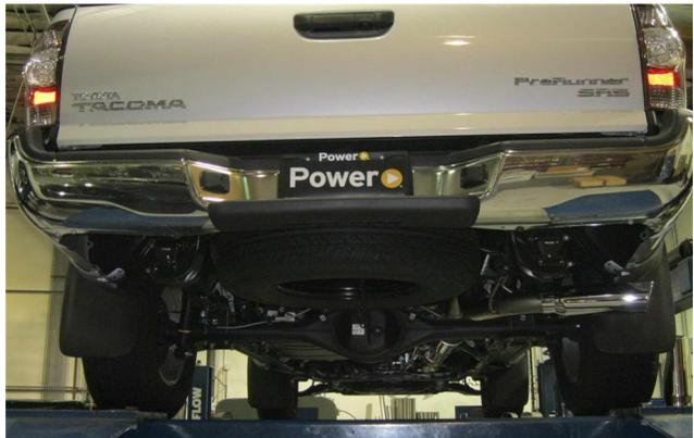
**Step 5.** Once a final position has been chosen for the new exhaust system, evenly tighten all clamps from front to rear using the torque specifications on page one of the instructions. Inspect all fasteners after 25-50 miles of operation and re-tighten if necessary.
