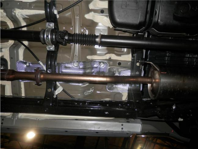
**Step 1.** Begin removal of the OEM exhaust system by unbolting the two bolts attaching the exhaust to the catalytic converter. Do not discard or damage the OEM fasteners or rubber insulators as they will be used to install the new system.
