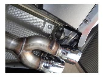
Step 3. Using the supplied rubber insulators install the Tailpipe Assemblies to the Muffler fitting the hangers into the installed hanger brackets. Install the bracket in between th two tailpipes.
