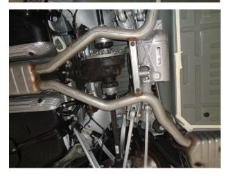
Step 1. To remove the OEM exhaust system, You can then disengage the welded hangers from the rubber insulators and remove the tailpipe assy. Unfasten the two brackets by the tailpipes, the clamp attaching the OEM inlet pipe assembly to the catalytic converter and the flange on the otherside. Do not damage or discard the inlet pipe clamp or rubber insulators as they will be reused to mount the new system. Disengage the inlet pipe assembly hanger and remove the exhaust from the vehicle.
