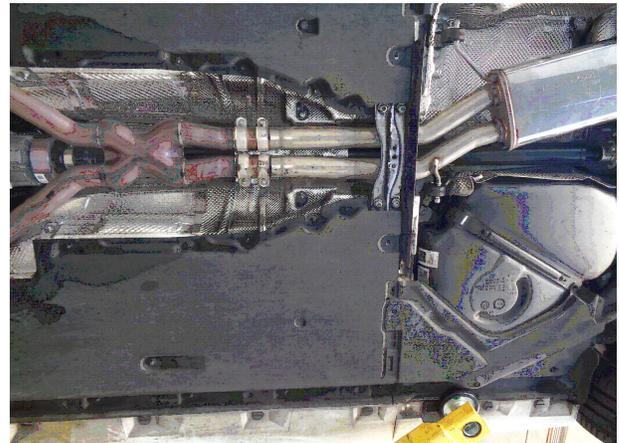
**Step 4.** Next attach the Resonator Assembly to the X-Pipe Assembly using the OEM clamps and fitting the hangers into the rubber insulators
