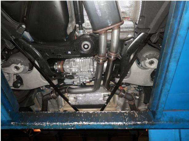
**Step 5.** Next attach the Mid Pipes to the outlets of the Resonator Assembly using the supplied V-Band clamps. **\*\*NOTE:** Take care when using the V-Band Clamps, they are designed for one time use only. Once the clamp is tightened it can not be reused.
