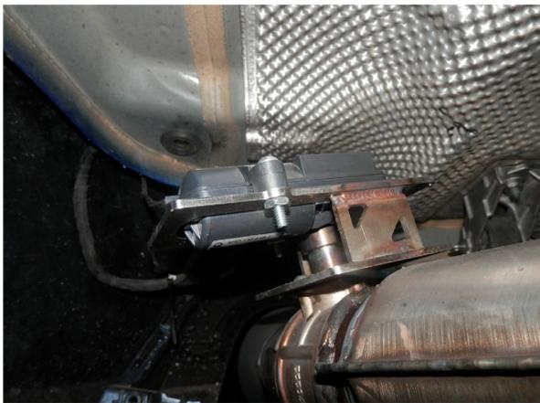
**Step 2.** Once the OE system is on the ground you will need to swap the servo motors from the factory control valves to the control valves on the Magnaflow Tip Assemblies. Use the new supplied hardware to attach the servo motors to the valves. At this point remove and retain the OE slip clamps to use on the new system.
