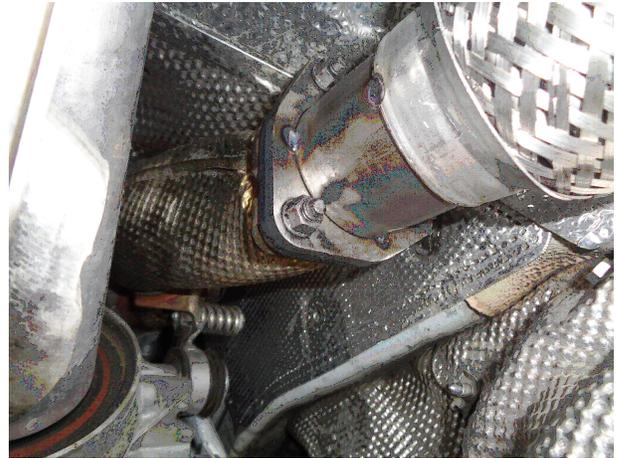
**Step 3.** Begin installation of the new system by fastening the X-Pipe Assembly inlets to the catalytic converter outlets using the OE fasteners (Leave all clamps and fasteners loose for final adjustment of the complete system.)
