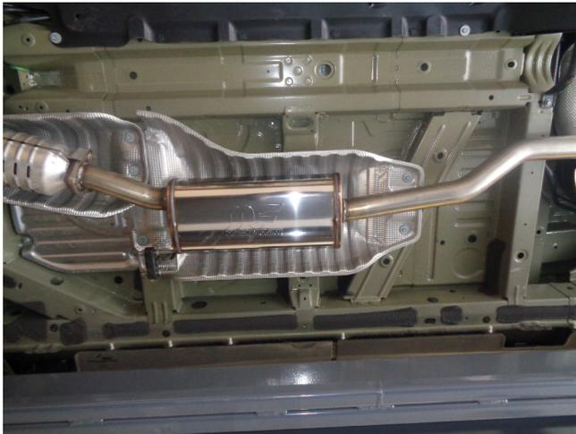
Step 2: Begin installing your new system by loosely bolting the inlet flange of the Muffler Assembly to the catalytic converter outlet using the OEM hardware. Engage both hangers to the rubber insulator.
