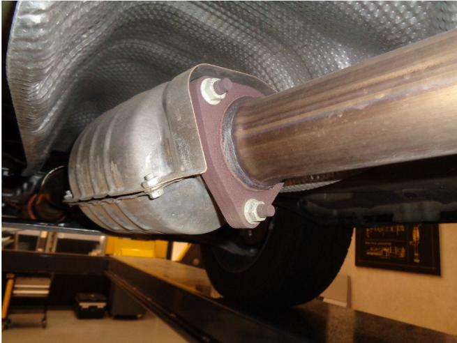
Step 1: To remove the OEM system first unbolt the inlet pipe at the catalytic converter flange junction. Working front to rear disengage all welded hangers from the rubber insulators. The OEM exhaust system may now be removed. Be sure to retain all mounting hardware as it will be needed to install your new MAGNAFLOW system
