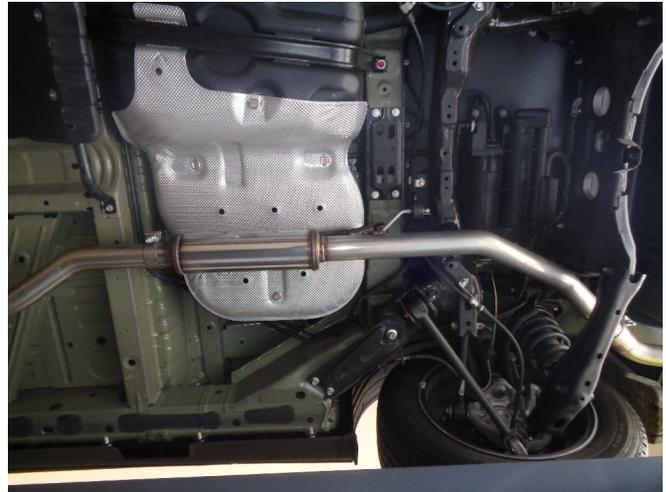
Step 3: Next loosely fasten the Resonator Assembly inlet to the outlet of the Muffler Assembly using the supplied clamp. Engage the welded hanger for the rubber insulator.
