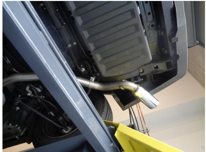
Step 4: Install the Tail Pipe Assembly in a similar fashion using the supplied clamp and engaging the welded hanger to the rubber insulator.
