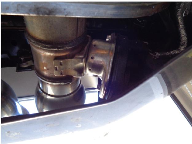
**Step 1.** To begin, determine if your vehicle has OE exhaust valves, if so, you will need to unplug the electrical connection on the Exhaust Valve Control Motors (Qty 2) located on the OEM exhaust assembly.
