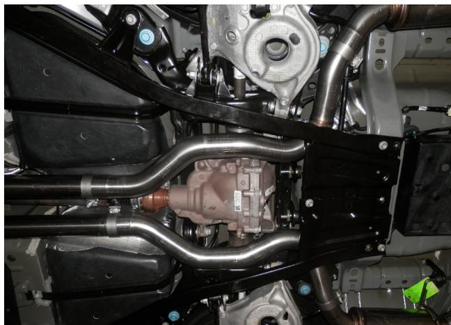
**Step 4.** Next attach the Mid Pipe Assemblies to the Resonator Assembly using the supplied 3.00" clamps and fitting the hangers into the rubber insulators.
