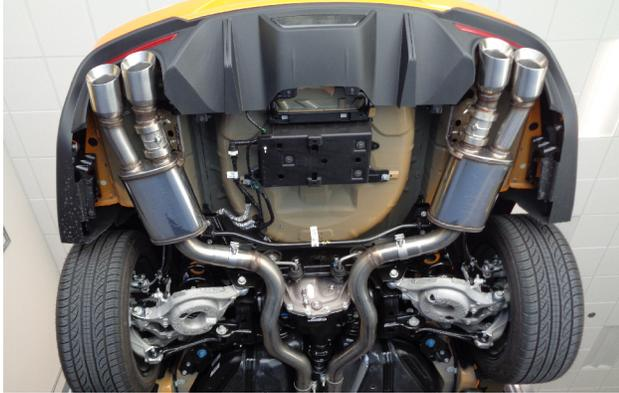
**Step 5.** Finish the initial installation by fitting the Muffler Assemblies onto the Mid pipe Assemblies using the supplied 3.00" clamps and inserting the hangers into the rubber insulators.
