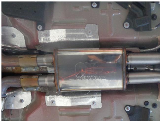
**Step 3.** Begin installation of the new system by loosely attaching the Resonator Assembly to the outlets using the OEM clamps. Leave all clamps loose until final adjustment.
