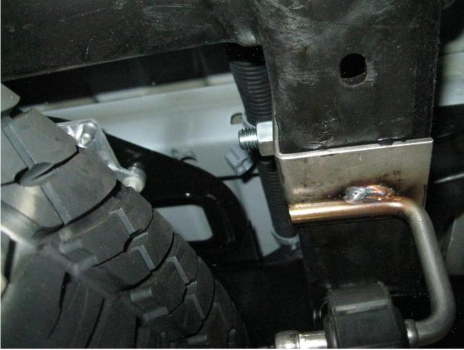
**Step 4.** At this point you will need to install the provided Hanger Bracket Assembly onto the D/S frame rail to allow for the installation of the dual system. Install the bracket to the frame rail with the supplied 1/2" fasteners and the backing plate for the backside of the rail. Fasten the Supplied Rubber Insulator to the hanger once mounted.
