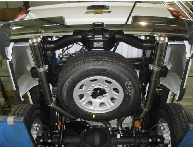
**Step 5.** Finish by installing the Tail Pipe Assemblies to the over axle Extension Pipe Assemblies and the Tips to the Tail Pipe Assemblies using the supplied 3.00" clamps and fitting the welded hangers into rubber insulators. Use the two  $\varnothing 3.00 \times 7.00$ " Extension Pipes between the Tail Pipe Assemblies and the Tips if your truck has a Long Bed configuration.
