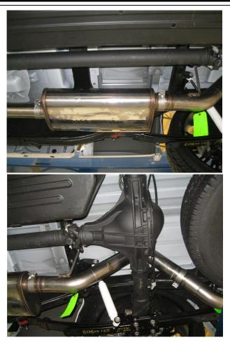
**Step 3.** Install the Muffler to the Inlet Pipe Assembly using the supplied 3.50" clamp. Next install the Over Axle Assembly to the Muffler in the similar fashion using the supplied 3.50" clamp, fitting the welded hangers into the rubber insulators.
