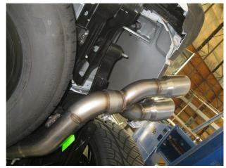
**Step 4.** Finish by installing the Tail Pipe Assembly to the Over Axle Assembly and Tip Assembly to the Over Axle using the supplied 3.50" clamps, fitting the welded hanger into rubber insulator.
