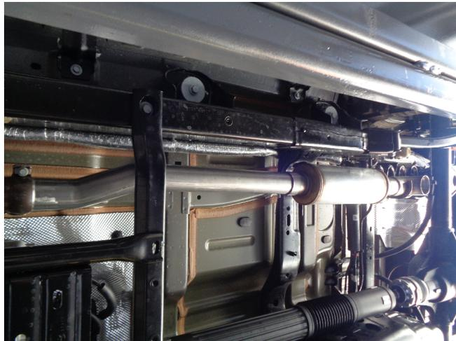
Step 3: Begin installation of your new MAGNAFLOW system by attaching the inlet assembly to the catalytic converter outlet using the OEM clamp. Keep all fasteners and clamps loose until final adjustment.
