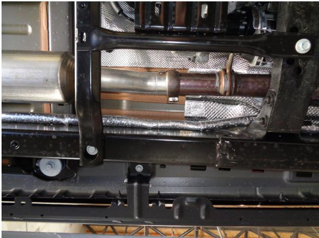
Step 1. Begin removal of the OEM exhaust system by loosening the clamp attaching the exhaust to the catalytic converter.
