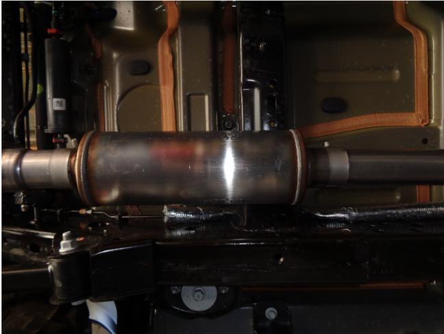
Step 4: Install the muffler assembly with supplied clamps along with the turn down pipe locating the rubber insulator.
