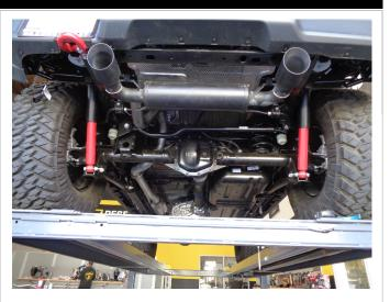
Step 2: Begin installing the new system by attaching the Muffler Assembly inlet to the OE outlet using the supplied 2.50 clamp. Engage the welded hanger to the rubber insulator. Keep all clamps and fasteners loose until final adjustment
