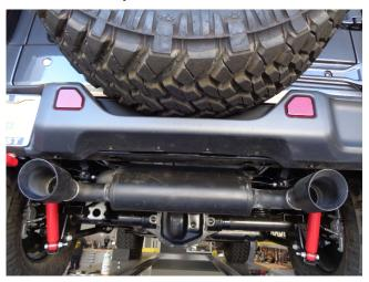
Step 3: Once a final position has been chosen for the new exhaust system, evenly tighten all clamps from front to rear using the torque specifications on page one of these instructions. Inspect all fasteners after 25-50 miles for operation and re-tighten if necessary.
