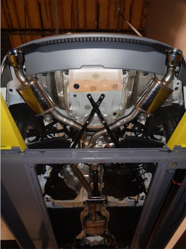
Step 4: Finish by attaching the driver and passenger side Muffler Assemblies to the Y-Pipe Assembly using the supplied 2.50" clamps and engaging the hangers to the rubber insulators. Reattach all braces.
