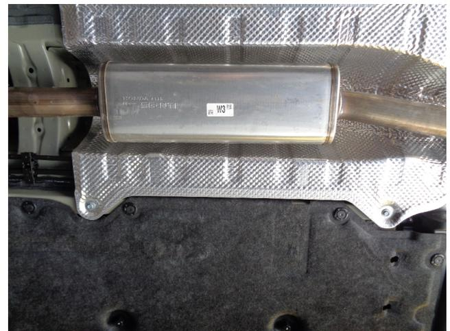
**Step 1.** To ease removal of the OE exhaust system unbolt the cross braces located on the underside the vehicle and remove. Begin by unfastening the rear muffler assembly at the flange located at the rear of the vehicle in front of the driver side muffler. Extract the hanger from the rubber insulators and remove the assembly. Do not discard or damage the OE fasteners or rubber insulators as they will be used to install the new system.
