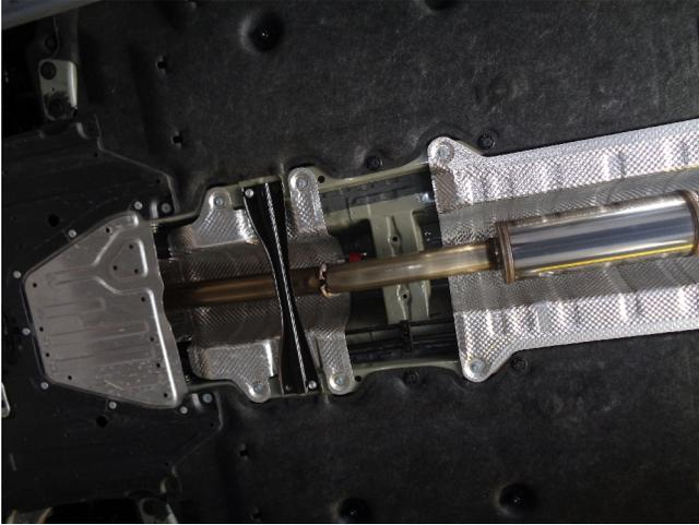
**Step 3.** Begin installation of your new MAGNAFLOW system by attaching the Resonator Assembly to the catalytic converter outlet using the OEM fasteners and insulator and the supplied ring gasket. Keep all fasteners and clamps loose until final adjustment.
