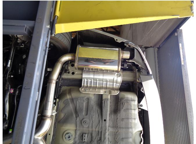
**Step 5:** Next use the supplied 2.50" clamps to attach the Muffler Assemblies to the Y-Pipe Assembly and insert the hangers into rubber insulators.
